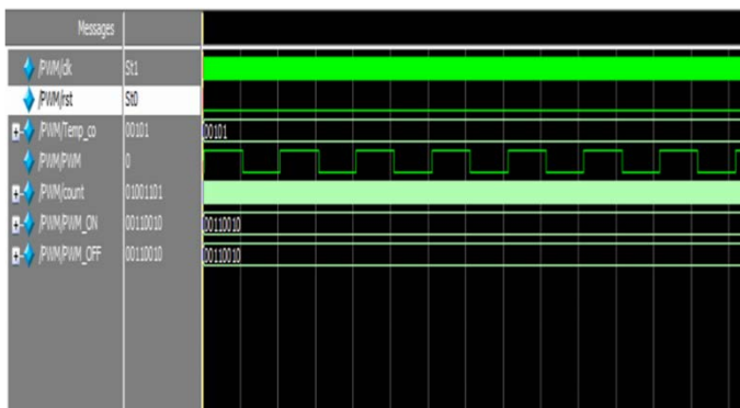
Fig.6. PWM pulses from the digital controller.
